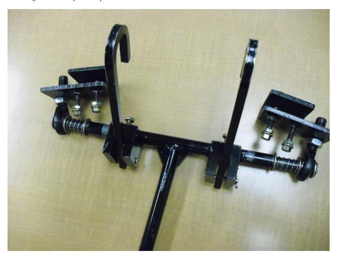
When the hand controls were ready, they were installed in the airplane. The special controls consist of two bracket clamps that attach to the pedals.
